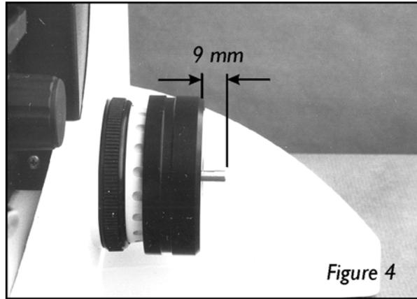
5. Fit the drive coupling on the fine focus shaft using the 1.5mm hexagonal wrench key. Orientate the shaft so that the grub screw will locate on the flat of the shaft. Push the drive coupling gently towards the adapter ring whilst tightening the grub screw. Check that the fine focus rotates freely and is still set at 1 micron.
