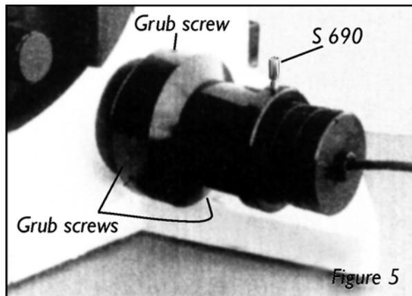
7. Slide the H249 Microstep Focus motor assembly into the motor sleeve and tighten the S690 thumb screw whilst gently pushing the focus motor assembly towards the microscope such that there is a good contact between the rubber surfaces of the drive of the motor and the drive coupling (figure 5). The fitting is now complete. The motor is now able to drive the fine focus mechanism of the microscope.
