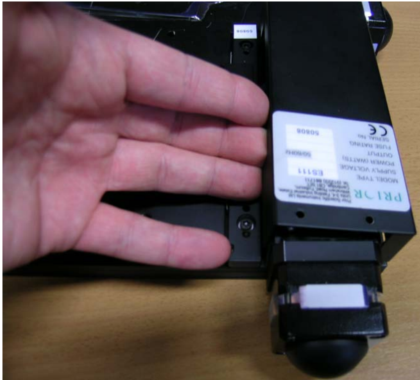
Figure b: Removal of Y-axis drive cover.
