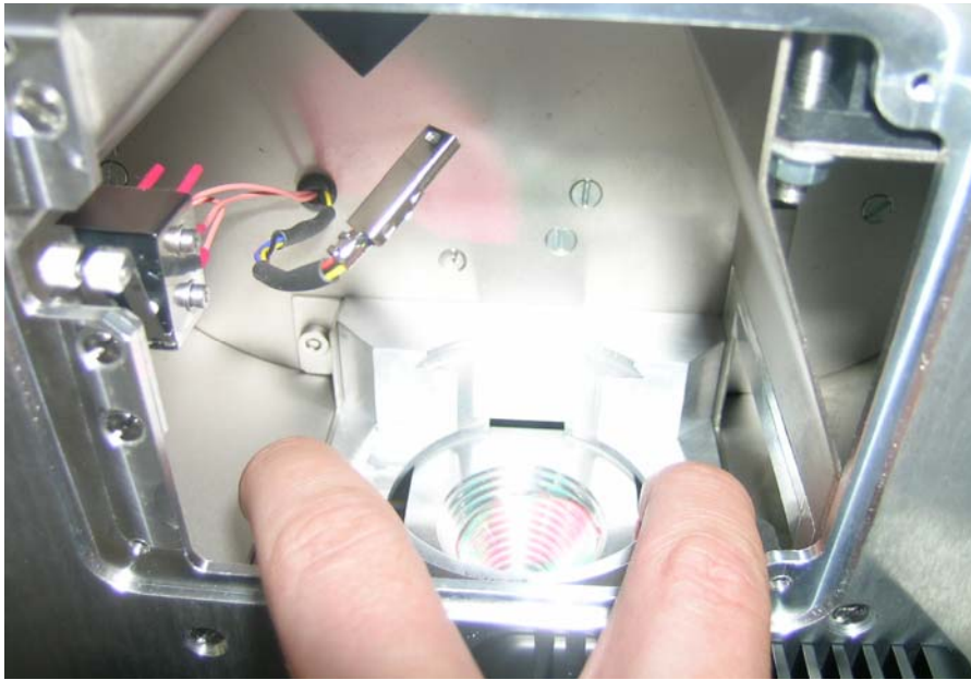
Figure showing the top section of the bulb clamp being pulled up with two fingers.
